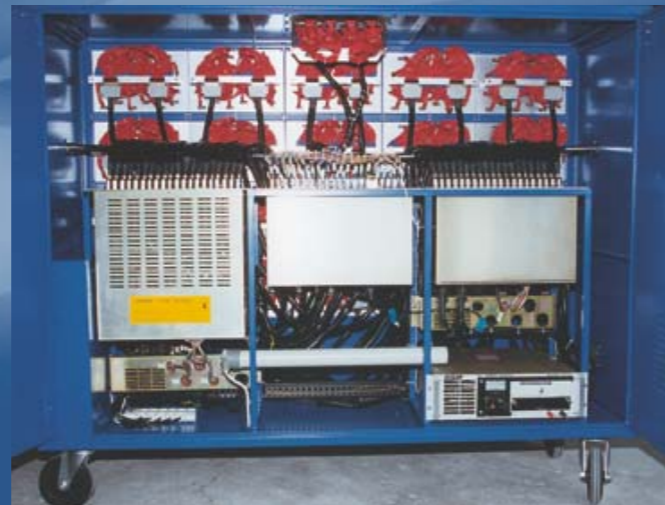
ACSR control consul for EH101 helicopter
