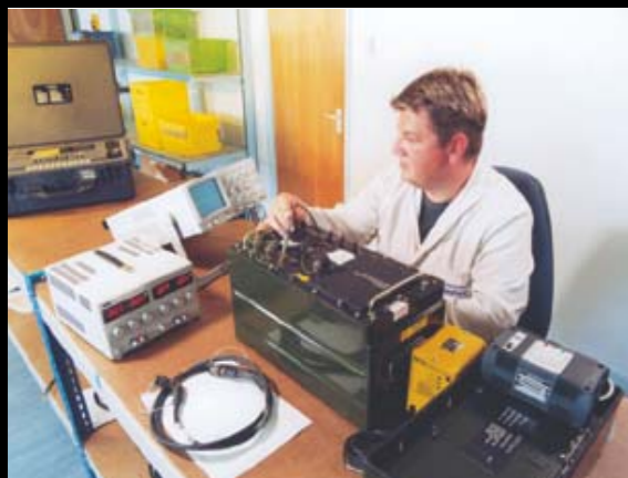
Computer controlled insulation & continuity testing system for aircraft wiring
