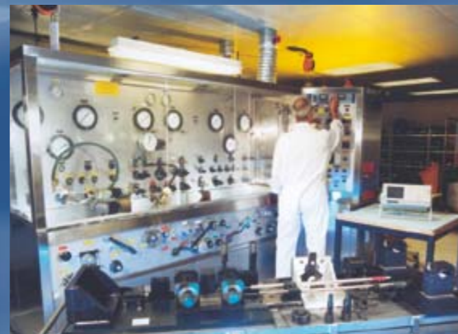
Test rig and tooling fixture for aircraft hydraulics
