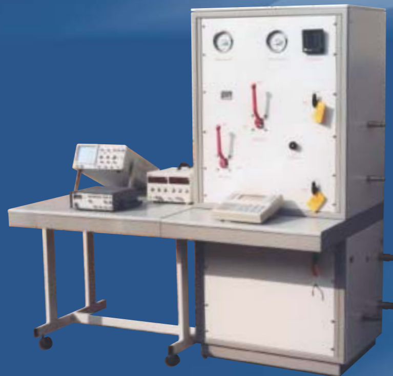
Calibration & test station for aircraft series actuators
